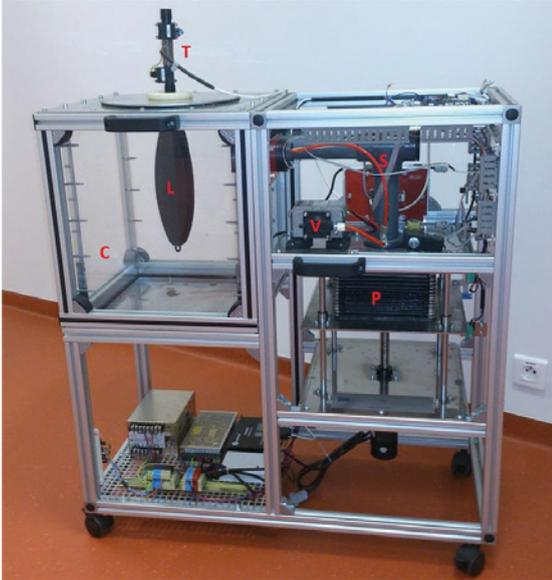
FIGURE 1 The electromechanical structure of the LUNG simulator [1]
